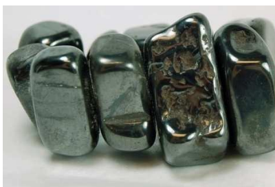
Above: example of a poor hematite tumble. These stones should not have left the First or Coarse stage!
